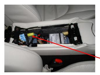
With Bluetooth, the PSEU (Portable Support Electronic Unit) will be connected to the yellow telephone harness connector.
