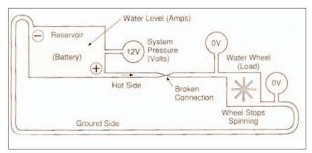
In this example, if the water pipe completely collapses, water stops flowing, pressure drops to zero and the water wheel stops turning. Electrically, the same thing happens when a wire falls off or a connection breaks. Current stops flowing, voltage drops to zero. A starter motor would quit or a head-light would go out.
