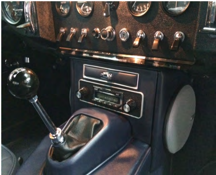
Period-looking radio is fully digital, IPod ready, yet no holes were cut. Even antenna isn't visible. New speakers in original locations.
