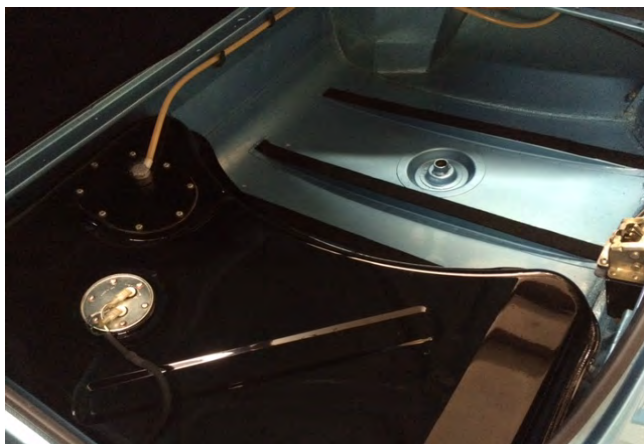
Refinished trunk floor, rub strips, fuel lines, and the world's most complicated gas tank shape. Ever.
