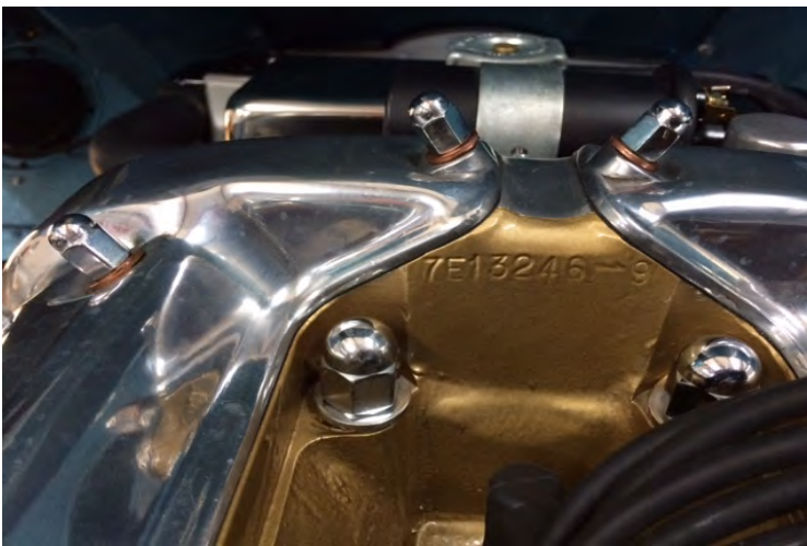
Engine number 7E 13246-9 from plate matches stamped number in head.
