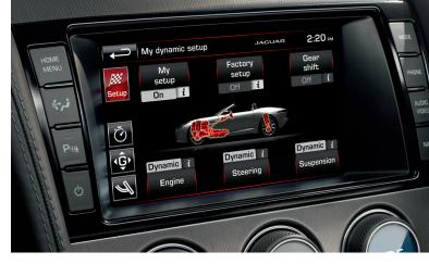
If your F-TYPE is fitted with Configurable Dynamics this can be set up to your own favoured dynamic driving settings using the configurable dynamics screen.
