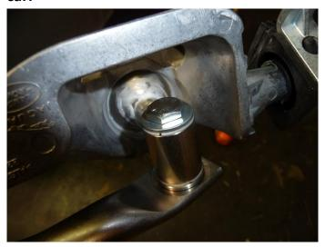
20. Fit all other parts back in reverse order, like exhaust shield, exhaust and shift boot/knob.
