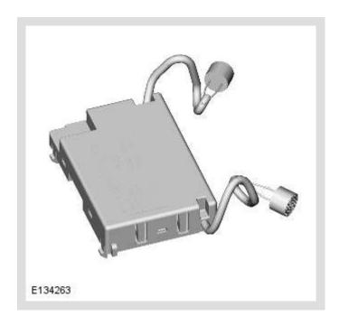
The volumetric sensor comprises two sensors which allow the interior of the vehicle to be monitored. The module is located in a central position in the front overhead console.
