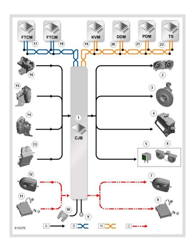
A = HARDWIRED CONNECTION; D = HIGH SPEED CAN BUS; N = MEDIUM SPEED CAN BUS; O = LIN BUS.
