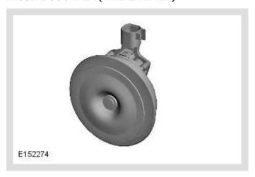
The passive sounder is located in the rear right corner of the engine compartment and attached to a bracket on the bulkhead panel. The passive sounder is connected directly to the CJB, which connects a power feed to the passive sounder when the alarm is triggered.
