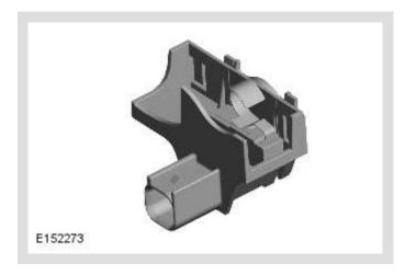
The hood switch is attached to the underside of the left hood latch and operated by movement of the latch mechanism. When the latch opens, the switch closes and connects a ground to the CJB.
