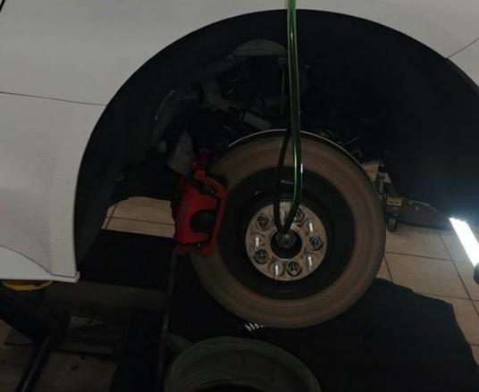
Once full, Use the same tools above and the same method to re-install the fill plug. Replace your wheel (*Don't forget to torque your lug nuts*!), and lower the car (unless you have AWD, and want to do the front!)
