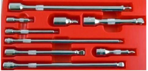
Various metric sockets, ratchets, extensions, long 3/8" extensions, a long 3/8" wobble extension, ball ended and regular ended Allen keys and sockets
