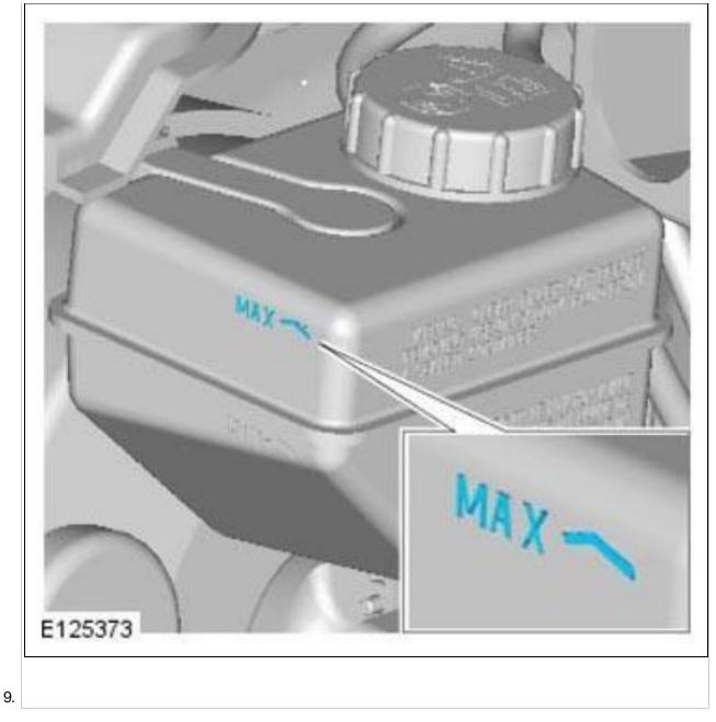
Fill the brake fluid reservoir to the MAX mark.
