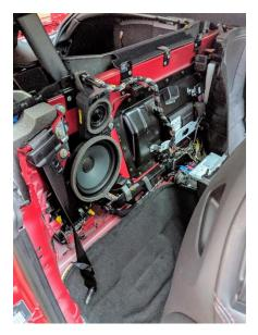
The picture on the left shows the rear speakers, the lower speaker is a 180cm subwoofer that is dual coil unit, and the upper speaker is a square unit that looks a bit like an oversized tweeter. Most people have avoided upgrading these units as they are very much custom for the F-type, and mounted in a moulded frame, which attaches to the bulkhead.
