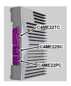
The first job is to create the loom to connect the speaker outs from the existing amplifier into the Audison. The amplifier has TE connectivity Multilock Hybrid (0.70,0.40) Connectors. However they are only available as wire to board configurations. So in other words you cant create a loom using these connectors as one end is designed to be mounted on a circuit board. So you will be cutting the loom!!
