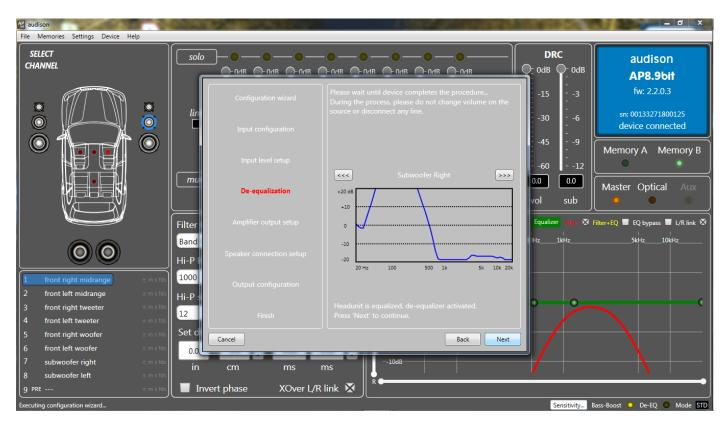
Once the tests are completed, you can then personalise the amp. The first step is to configure the output. For my design, that is 3 way at the front plus left and right subs that are mounted in the rear. After you have completed the configuration wizard, you can then plug the speakers back in and start to tune the system.
