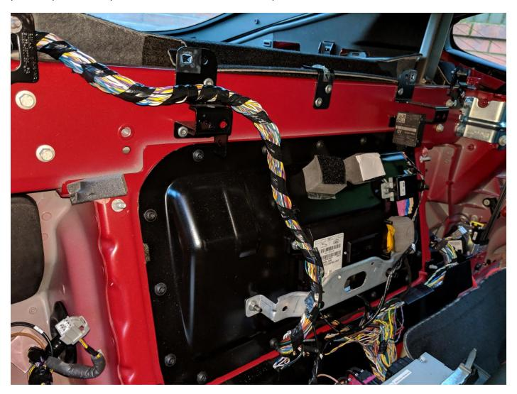
This is a point to note as the coupe has its amplifier tucked away behind the rear bulkhead below the rear quarterlight on the right-hand side of the car. The convertible amp is mounted in the centre of the front of the rear bulkhead.
