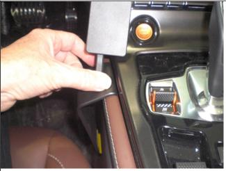
1. Peel off the cover of adhesive tape on the ProClip. Note: The adhesive tape does not leave any marks or damage the dashboard, and is easy to remove. Place the ProClip in your hand so the ProClip label (sticker) is in an upright position, or if vertically positioned; the P in ProClip is at the top.
