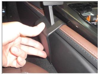
2. Press downward on the ProClip so the lower angled edge hooks under the lower section of the console sidewall.
