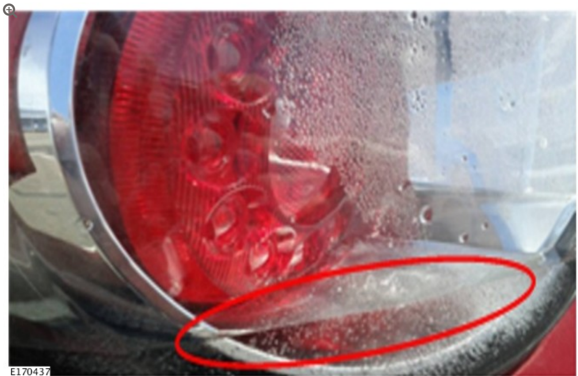
Standing water within the lamp.
