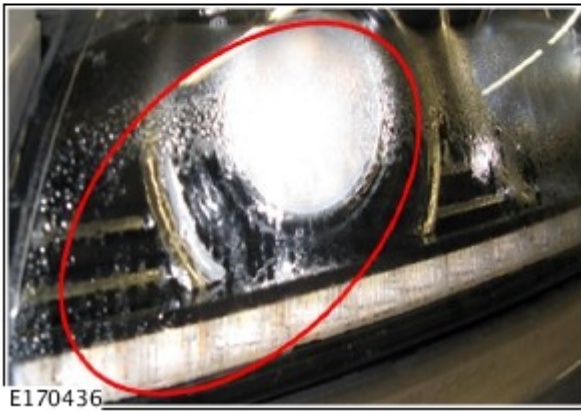
Drip marks or streaks in the condensation.
