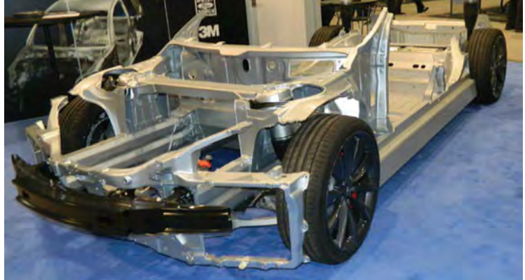
This Tesla chassis is all aluminum, and structural repair parts are restricted to approved shops. It was on display at the SEMA Show by SCRS.
