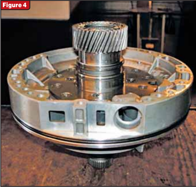
Pump showing how the front planetary sun gear is held stationary
