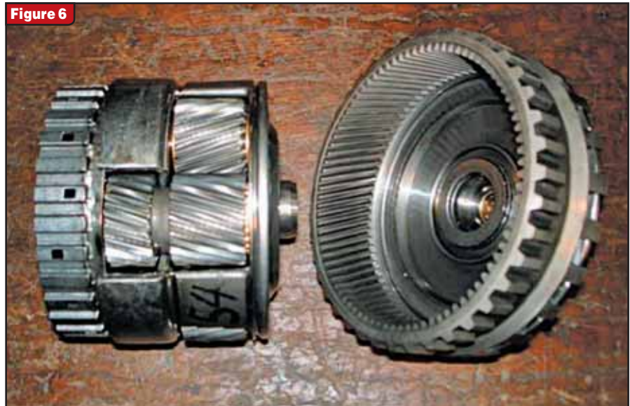
The Lepelletier gear train
