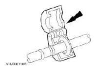
3. Close the special tool and push it into the female end of the spring lock coupling.
