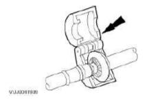
6. Connect the spring lock coupling.
