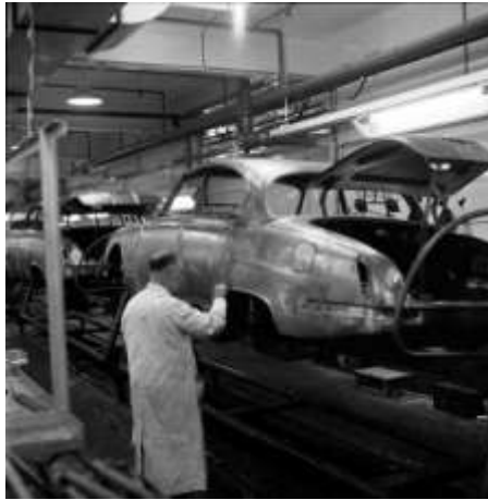
Inspecting the degreased 'S'-type bodyshell.
