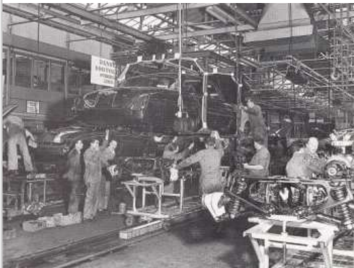
An 'S'-type bodyshell being lowered onto the car's 'skeleton' on the Main Assembly track. Note: Mk2 line in background,
