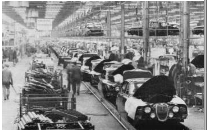
Two views of the 'S'-type production area, Note the overhead Body Assembly track feeding bodyshells to the lower Main Assembly Track.
