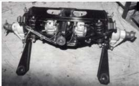
'S'-type subframe-mounted rear suspension of the 'S'-type. Note: for a wire wheeled car.
