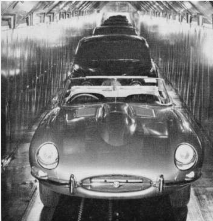
Completed 'S'-types, behind an E-type, coming through the drying oven following the final 'top coat' applied after final test.
