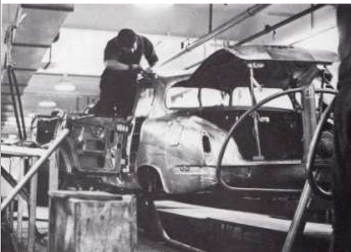
Minor defects are rectified before priming and painting. Fit of doors, bonnet and boot lid are also checked at this stage.
