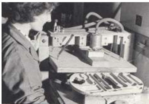
'S'-type toolkit base being cut on a rotor machine.
