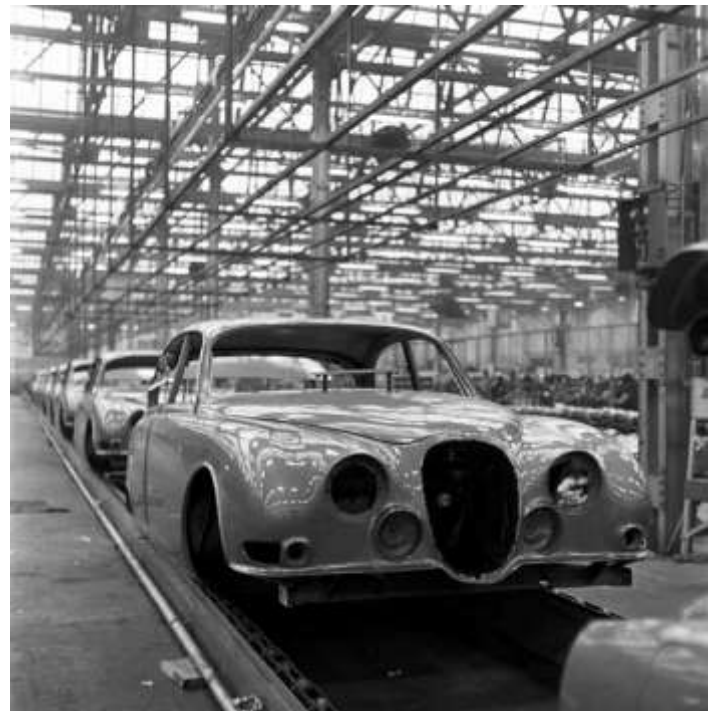
Minor defects are rectified before priming and painting. Fit of doors, bonnet and boot lid are also checked at this stage.
