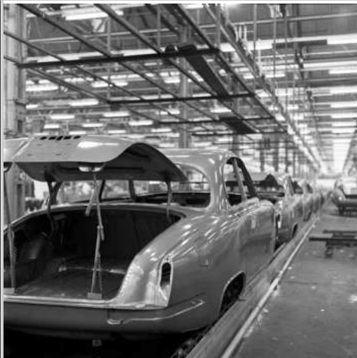
Above and previous page, Finished painted 'S'-type bodyshells moving to join the Main Assembly Track.
