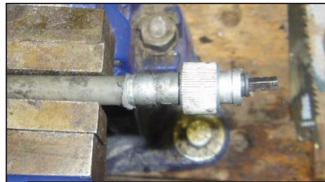
Figure 4: The completed cable, Jaguar end.
