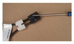
Using the same screwdriver, or other small implement, release the individual cable end from the housing by **GENTLY** lifting the plastic clip on the top which secures it within the plug.
