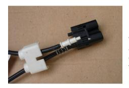
Do the same on each new or additional cable you wish to add to the ring – you should be displacing an IN cable on one side and on the other connector an OUT cable to maintain a one way flow around the ring
