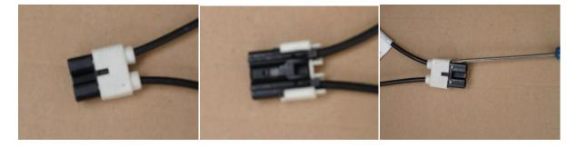
Use a small flat blade screwdriver to remove the white plastic clip from the fibre connector by gently prising the sides and pulling the clip down at the same time.
