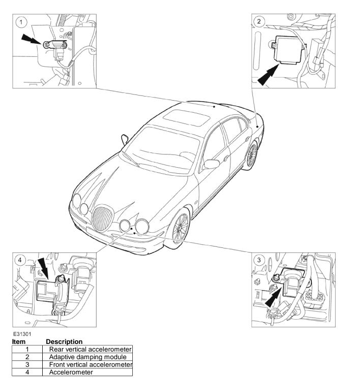
The vehicle dynamic suspension system is designed to control excessive body motions in bounce, pitch and roll while maintaining/improving ride and feel. The system controls the settings of the four vehicle dampers between firm and soft based on the road conditions and driver inputs.
