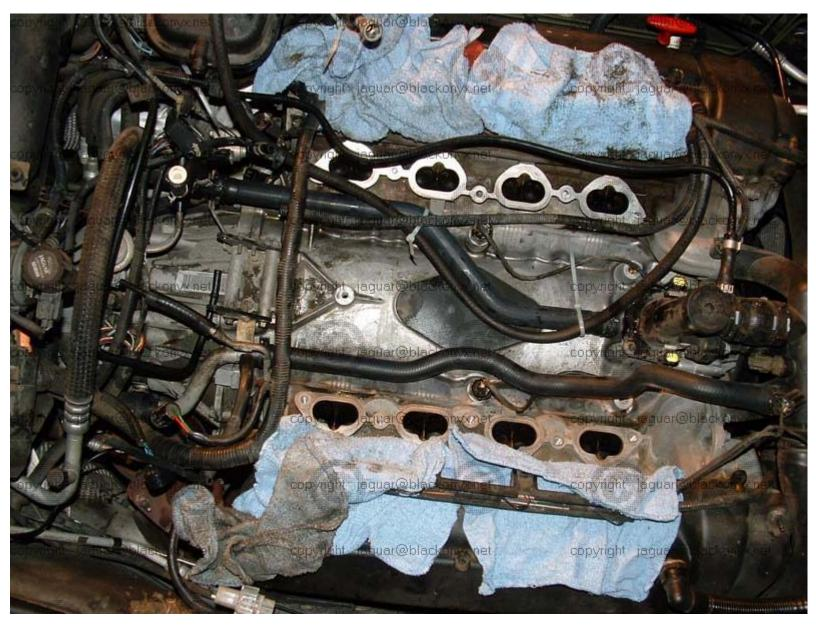
19) Once you have the hoses installed properly clean all the gasket surfaces. This includeds both sides of the intake ports, the elbow surface and the throttle body surface. Be careful not to scratch the surfaces.
