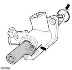
23 . **NOTE:** Ensure that the rack bar to rack housing orientation marks made at step 6 are aligned before attempting to install the pinion housing.
