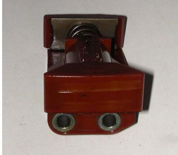
Fig. 10 Slipper surface showing minimal wear
