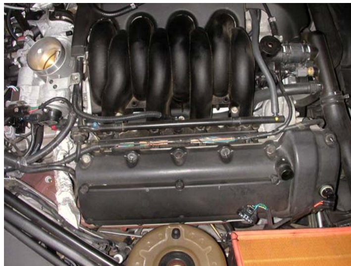
Fig. 4 Right-side view of engine bay with intake tube and right-side engine cover removed. Note the air filter and body are still in place.
