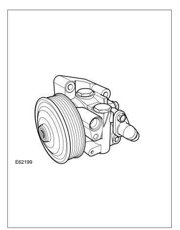
A variable displacement power steering pump has replaced the previously fitted fixed displacement power steering pump.
