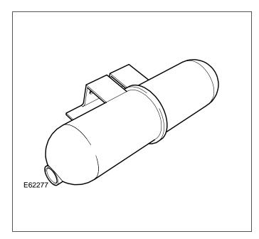
A secondary air injection vacuum reservoir is located on the right-hand side of the engine bay. The secondary air injection vacuum reservoir is included in the vacuum supply line between the intake manifold and the secondary air injection vacuum solenoid valve.
