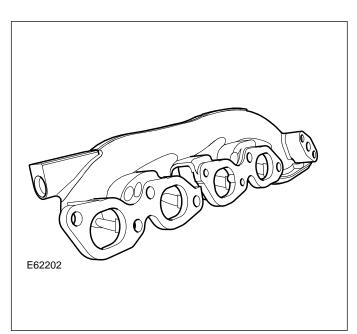
Due to the introduction of secondary air injection, this vehicle has been fitted with revised exhaust manifolds.
