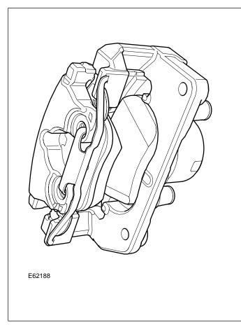
With the increased caliper piston size, the brake discs have also been enlarged from 300 mm to 326 mm.
