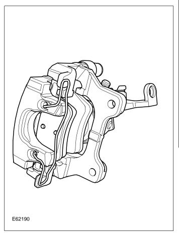
There is now only one size of brake disc available for foundation level brakes at 326 mm.
