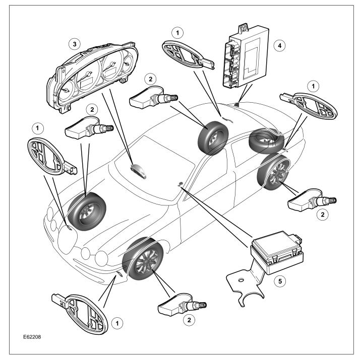
Tire Pressure Monitoring System - Component Location
