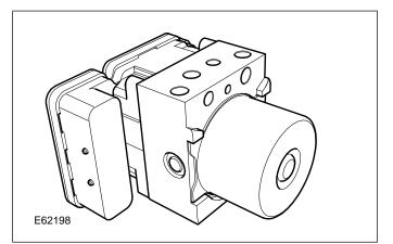
This model year (MY) vehicle sees the introduction of two variants of the hydraulic control unit and anti-lock brake system (ABS) module. The two hydraulic control unit and ABS modules are for non-adaptive cruise control (ACC) and ACC equipped vehicles.
