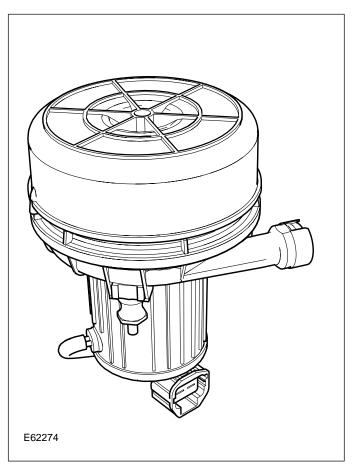
The secondary air injection pump is located behind the left-hand side of the front bumper cover. The pump is fitted on rubber mountings to help suppress noise generated by secondary air injection pump operation. The secondary air injection pump is powered from the battery by a dedicated relay and supplies approximately 10-15 kg/hr (22-33 lb/hr) of air when the vehicle is at idle on initial start up from 20°C (68°F).
