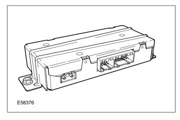
The voice activated control module is fixed to a bracket which also supports the PSE and the navigation control module.
