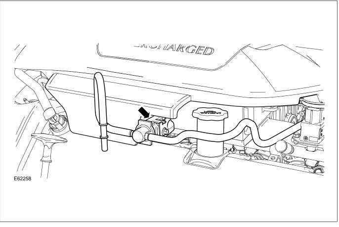
The Engine Control Module (ECM) operates the valve to purge fuel vapor from the evaporative emission canister into the engine for combustion. Purge rates (the extent that the purge valve opens) are determined by the engine operating conditions and the vapor concentration level. The purge rates are adjusted to maintain vehicle, driving characteristics and exhaust emissions at optimum levels.
