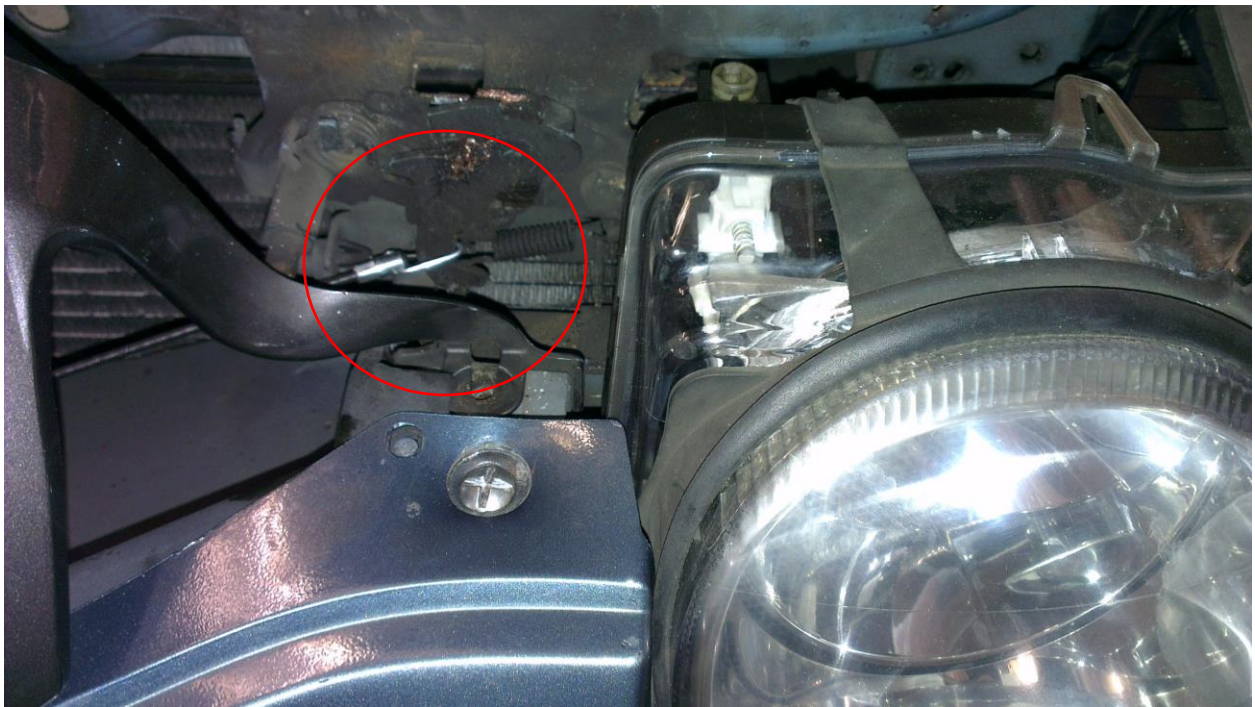
Hooked nail pulling on the latch release arm
