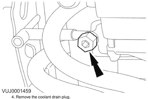
• Drain the coolant into a suitable container.
