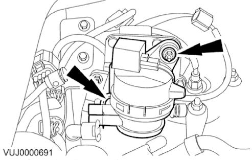
3. Remove the canister purge valve.
