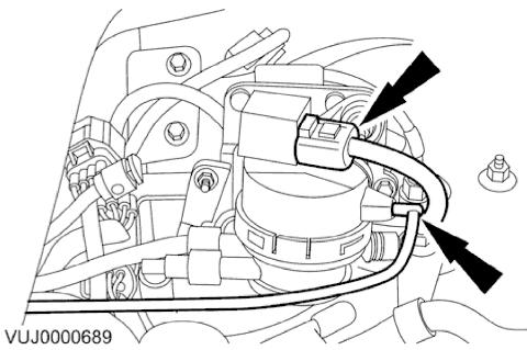
1. Disconnect the canister purge valve electrical connector and vacuum hose.
