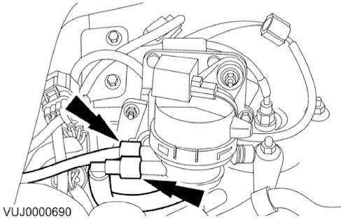
2. Disconnect the canister purge valve vacuum hoses.
