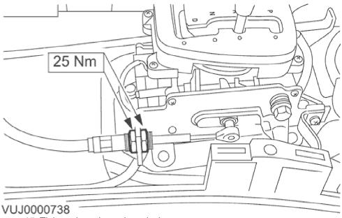
15. Tighten the selector lever lock nut.
