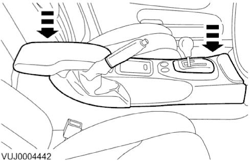
18. Install the center console upper section.
