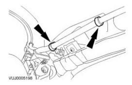
19 . Remove the roof opening panel rear drain hose.
