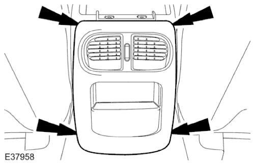
11. Release the floor console rear air register trim panel retaining tangs.
