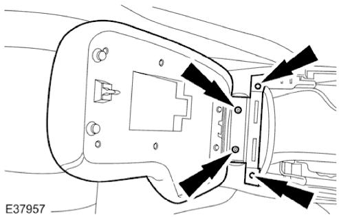
9. Remove the floor console glove compartment lid.
