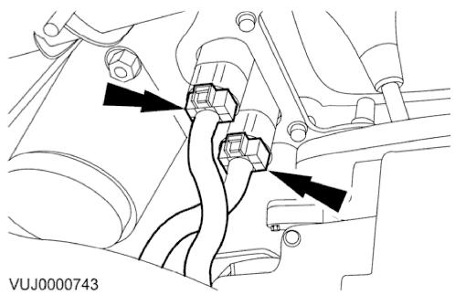
5. Disconnect the transmission mode, traction control and cellular phone electrical connectors if equipped.
