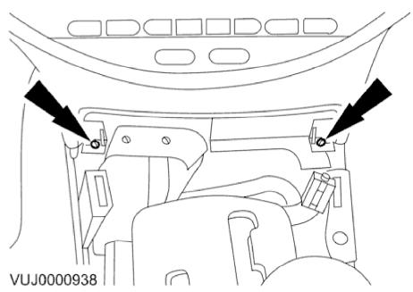
10. Remove the floor console front retaining screws.
