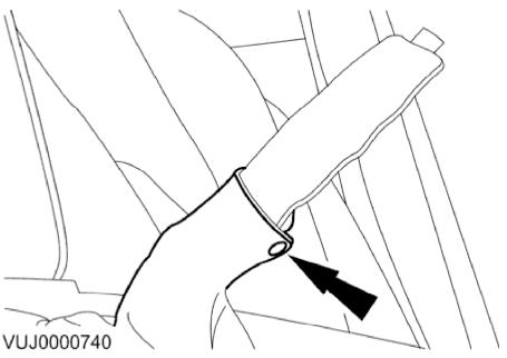
2. Release the parking brake boot retaining clip.
