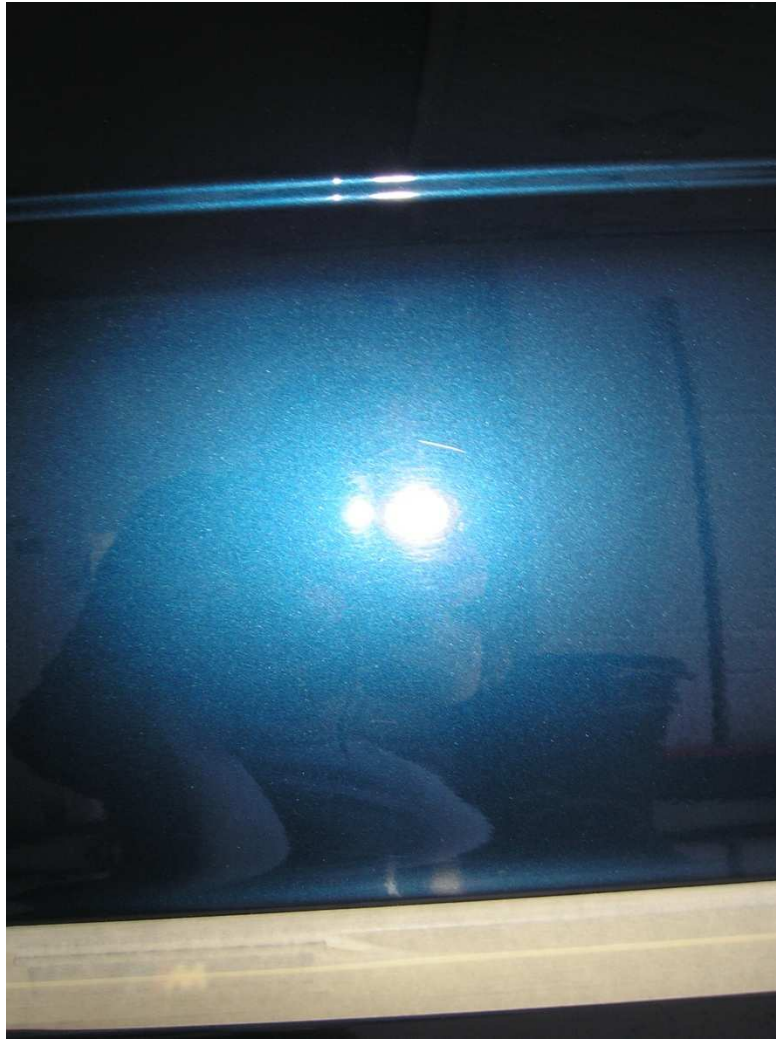
Light swirls removed, but more severe marks still remaining
