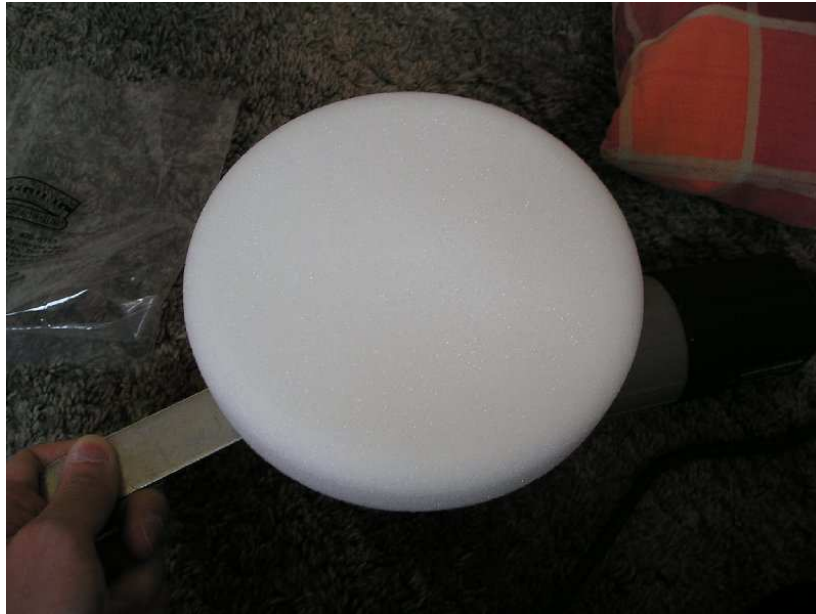
Holding bolt still, tighten backing plate to secure it to the machine
