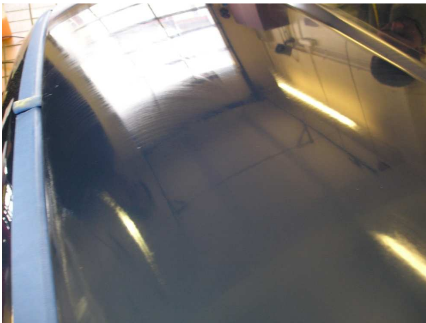
Fully broken down polish shows a clear, thick water like residue
