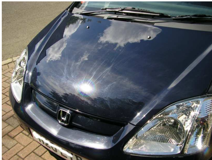
Holograms (from previous poorly finished machine polishing)
