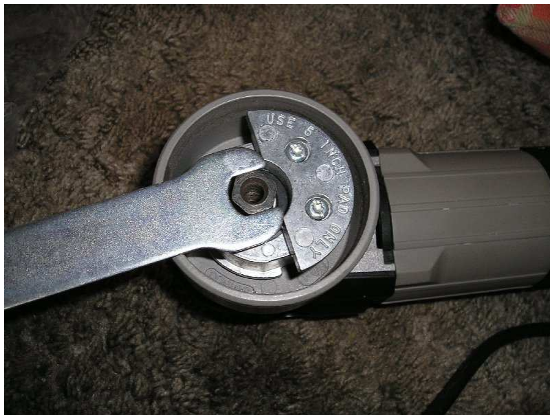
Holding the bolt still to securely fit the backing plate
