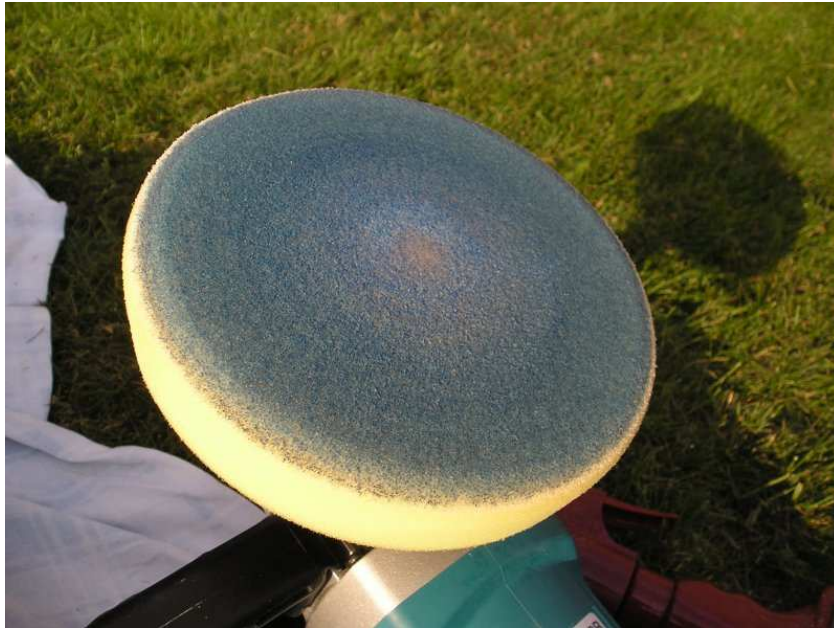
Pad stained by colour coat after clear coat strike through
