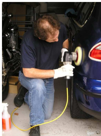
PC with 6” Pad (Meguiars W8006)
