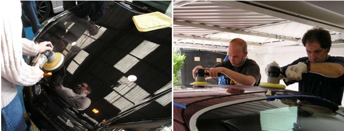
Left: Using a PC7424 with no handle Right: Using a PC7424 with a handle
