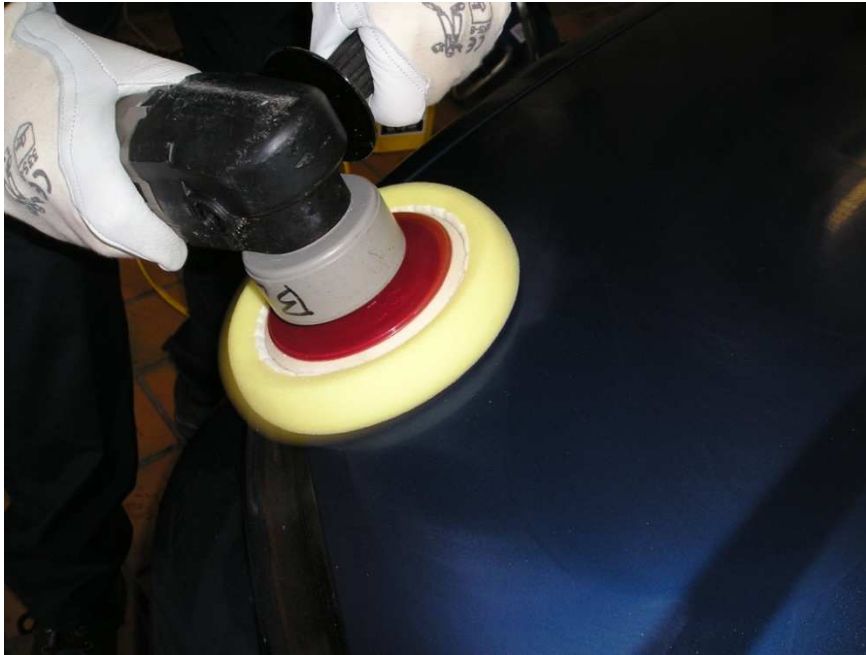
Working a polish using the Porter Cable 7424
