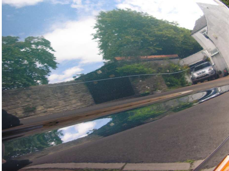
Deep scratch clearly visible in Jaguar S-Type paintwork
