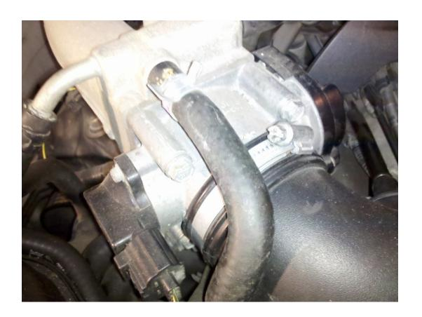
Disconnect vacuum tube from air intake hose
