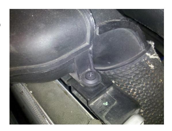
Remove 6mm air filter box fixing bolt (10mm socket w/extension)
