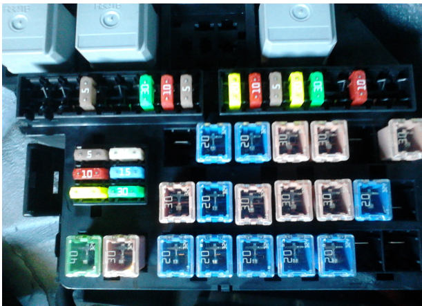
Rear Power Distribution Fuse Box (at left) showing vacant #8, #9 at lower right end; and #38, #39 at upper right end ... although any post connected directly to BATT POS will be suitable for installation of 10A fuse required for permanent connection of charger lead. Pic (at right) shows charger lead passing into locked boot/trunk, over soft, spongy dust seal.
