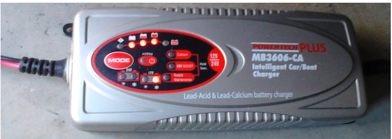
Powertech Plus 7A "intelligent" charger at work. Lower LED indicates it is set to Mode 4 at 14.7V while upper LEDs indicate that at 75%, "bulk" charge is now switching to "trickle". A final top LED will light or flash forever as charge moves in and out of "maintenance mode".
