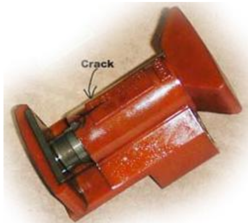
This tensioner is cracked in the typical way first-generation tensioners fail. Cracked tensioners can break apart, causing severe engine damage.
