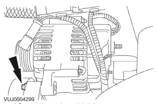
6. Remove the generator lower retaining bolt.
