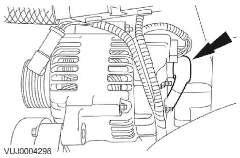
3. Detach the generator battery positive cable protective cover.
