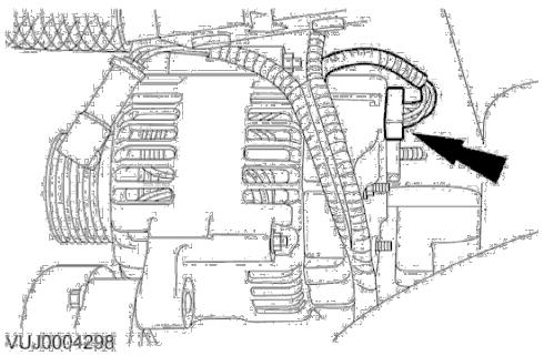
5. Disconnect the generator electrical connector.
