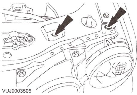
Adjust the headlamp using the adjustment bolts.
