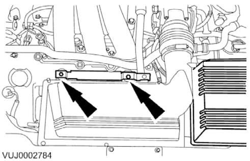
4. Remove the engine cover mounting plate.
