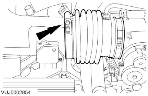
3. Disconnect the air cleaner outlet pipe.
