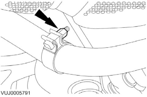
2. Loosen the rear muffler exhaust clamp nut.
