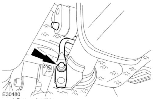
2. Tighten bolt to 25 Nm.
