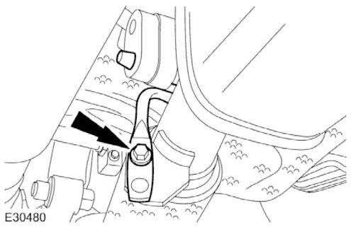
3. Detach the front muffler exhaust hanger isolator bracket.
