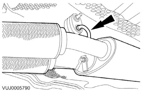
5. Detach the front muffler exhaust hanger isolator.
