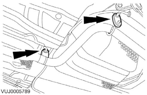
6. Detach the front muffler hanger isolators.
