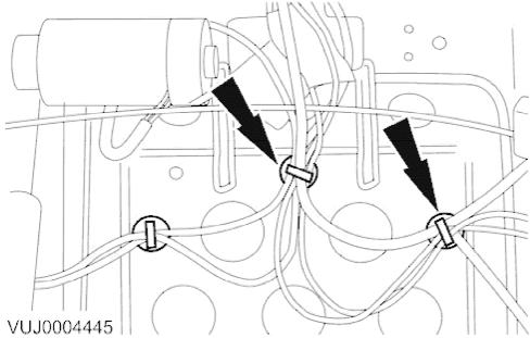
5. Detach the safety belt buckle and pretensioner wiring harness.
