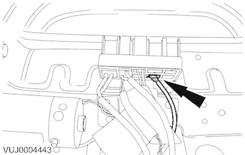
3. Disconnect the safety belt pretensioner electrical connector.
