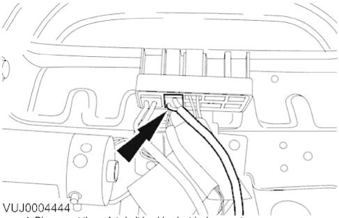
4. Disconnect the safety belt buckle electrical connector.
