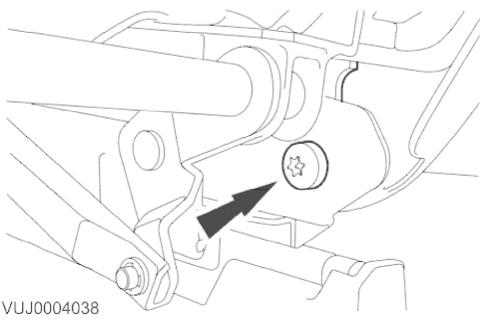
5. Detach the safety belt lower anchor from the underside of the seat.
