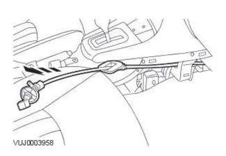
14. Lower the vehicle.15. Remove the selector cable.
