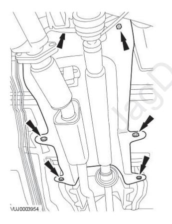
10. Remove the gear selector cable shield.
