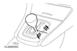
Using the corner of the grey feature line that follows the edge of the 'J' gate as a datum, use a rule and move the gear selector forwards or back two millimeters.
