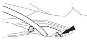
7. Detach the gear selector cable grommet.
