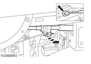
5. Detach the gear selector cable from the J-gate.
