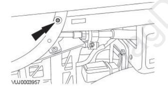
4. Remove the center console side retaining screw.
