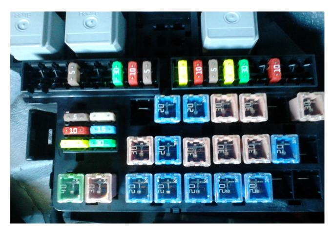
Rear Power Distribution Fuse Box in 2007 S-Type with 40A Fuse #1 at lower left corner.
