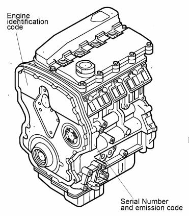
The production fit Puma diesel engine Serial number is 12 digits long and denotes engine capacity and date in reverse order
