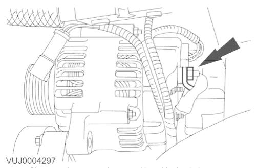
4. Disconnect the generator battery positive cable electrical connector.
