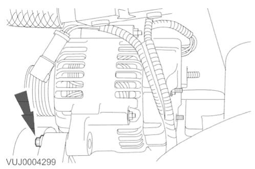
6. Remove the generator lower retaining bolt.
