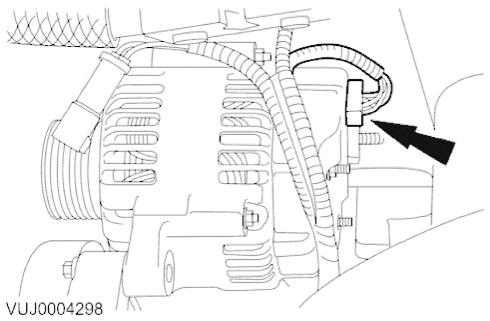
5. Disconnect the generator electrical connector.
