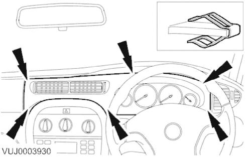
3. Remove the instrument cluster and vent finish panel.
