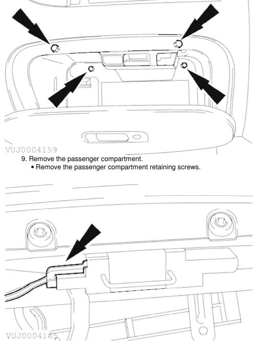
10. Disconnect the passenger compartment lamp electrical connector.
