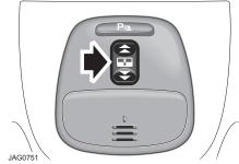
The sunroof is fitted with a facility that allows it to be fully opened or closed with a single operation of the indicated switch.
