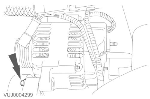
6. Remove the generator lower retaining bolt.
