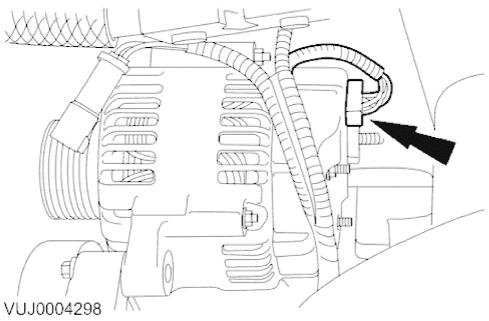
5. Disconnect the generator electrical connector.
