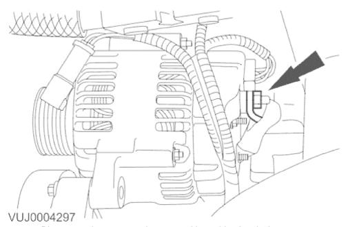
4. Disconnect the generator battery positive cable electrical connector.
