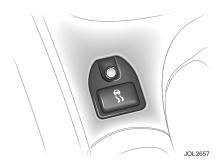
Dynamic stability control is operational whenever the engine is running, unless it has been switched off. If the system is operating, the warning light in the instrument panel will flash.
