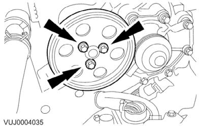
5. Remove the water pump drive pulley.
