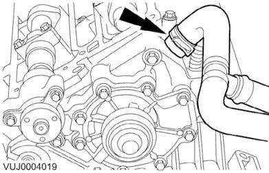
6. Detach the coolant expansion tank outlet hose from the water pump housing.
