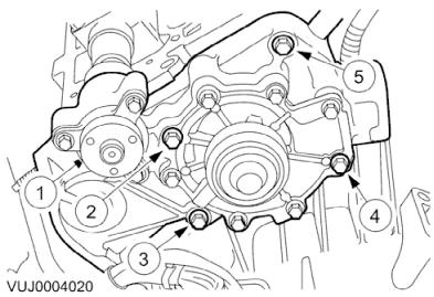
Make sure that the water pump housing is tightened in the sequence shown. Failure to follow this instruction may result in damage to the water pump drive pulley bearings.
