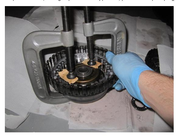
12. Remove the spring retainer and the spring underneath.
