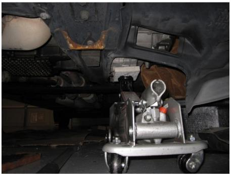
4. Remove the air filter, battery, and battery tray to expose the driver's side engine mount. Remove the engine mount through bolt. This might cause the engine/tranny to shift a bit.
