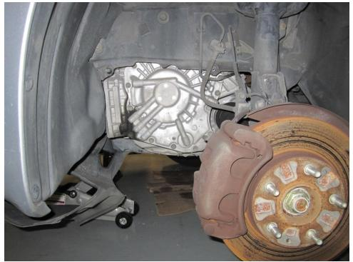
3. You will need to lower the engine & transmission a bit in order to fully access the end panel. Make sure your engine/transmission is supported. Since the engine mount member is still supporting the transmission, a jack may not be necessary, but I felt better with it in place. I originally had the jack on the oil pan, but found that wasn't far enough over on the driver's side to effectively lower/raise the transmission. I placed it on the driver's side of the engine mount member.
