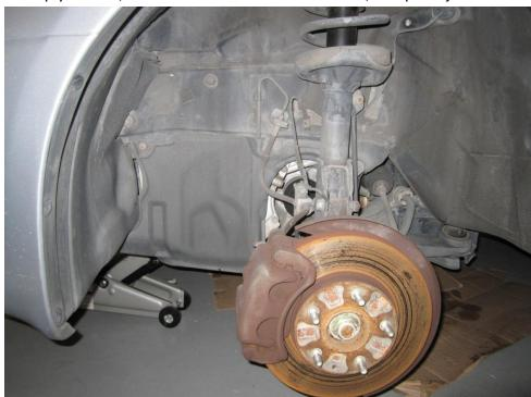
2. Remove the nut, bolt, and plastic body fastener, and fold the plastic splash guard forward, exposing the transmission end panel.
