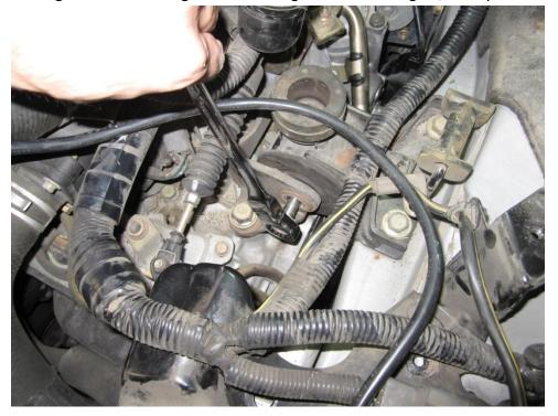
5. Loosen, but don't remove, the 3 bolts (2 front, 1 rear) on the engine mount member to allow the engine/ transmission to lower some. Even with the jack supporting the transmission, be careful here- there's not much supporting the driver's side of the transmission at this point.
