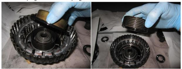
13. Remove the reverse and high pistons from the drum. To do this, place the clutch drum back in the end cover that you took off the transmission housing. Using compressed air, blow air into the proper hole to get the pistons to pop out. Take a break- now you've got the thing disassembled!
