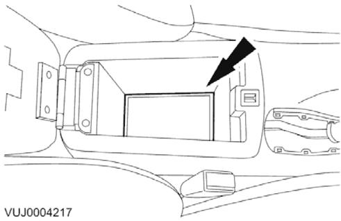
4. Remove the console stowage compartment non slip mat.
