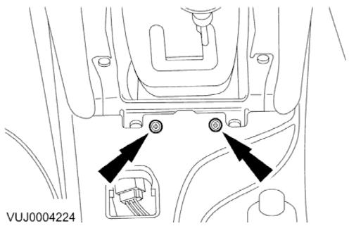
11. Remove the retaining screws.
