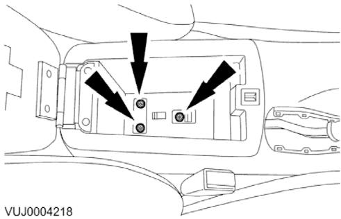
5. Remove the retaining screws.
